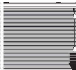
To Raise: Pull The Cord Straight Down With Short Strokes.
